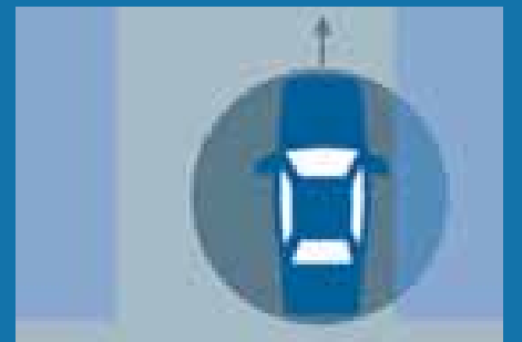
3. Now the vehicle position has been determined accurately and is updated constantly, whereby the system compares all the sensor data with the information on the digital map.
