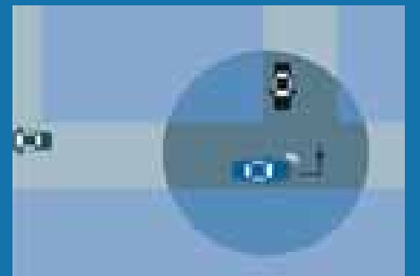
2. After just a few meters, the road the vehicle is traveling on can be identified. Any turns are recorded by the gyroscope.
